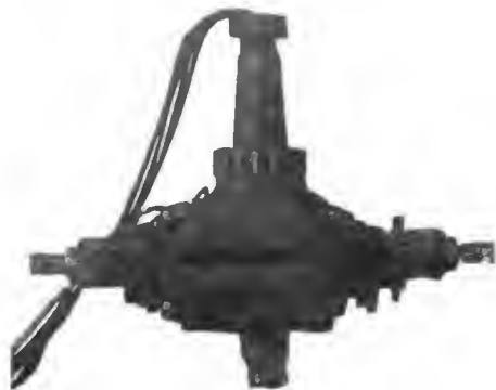
HUB MOTOR, SHOWING STUB JOURNAL AND WIRES, ROLLER BEARING AND DRIVE EQUALIZER.
